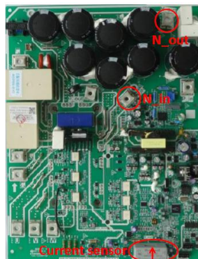
Figure 6-2.5: DC detection wire connection method
